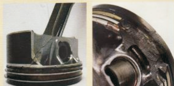
Two examples of piston damage due to LSPI observed during testing at Southwest Research Institute® Photo courtesy Southwest Research Institute®
